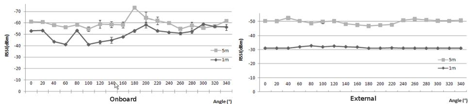
**Figure 1:** Average RSSI at a distance of 1m and 5m with one node equipped with an external antenna
